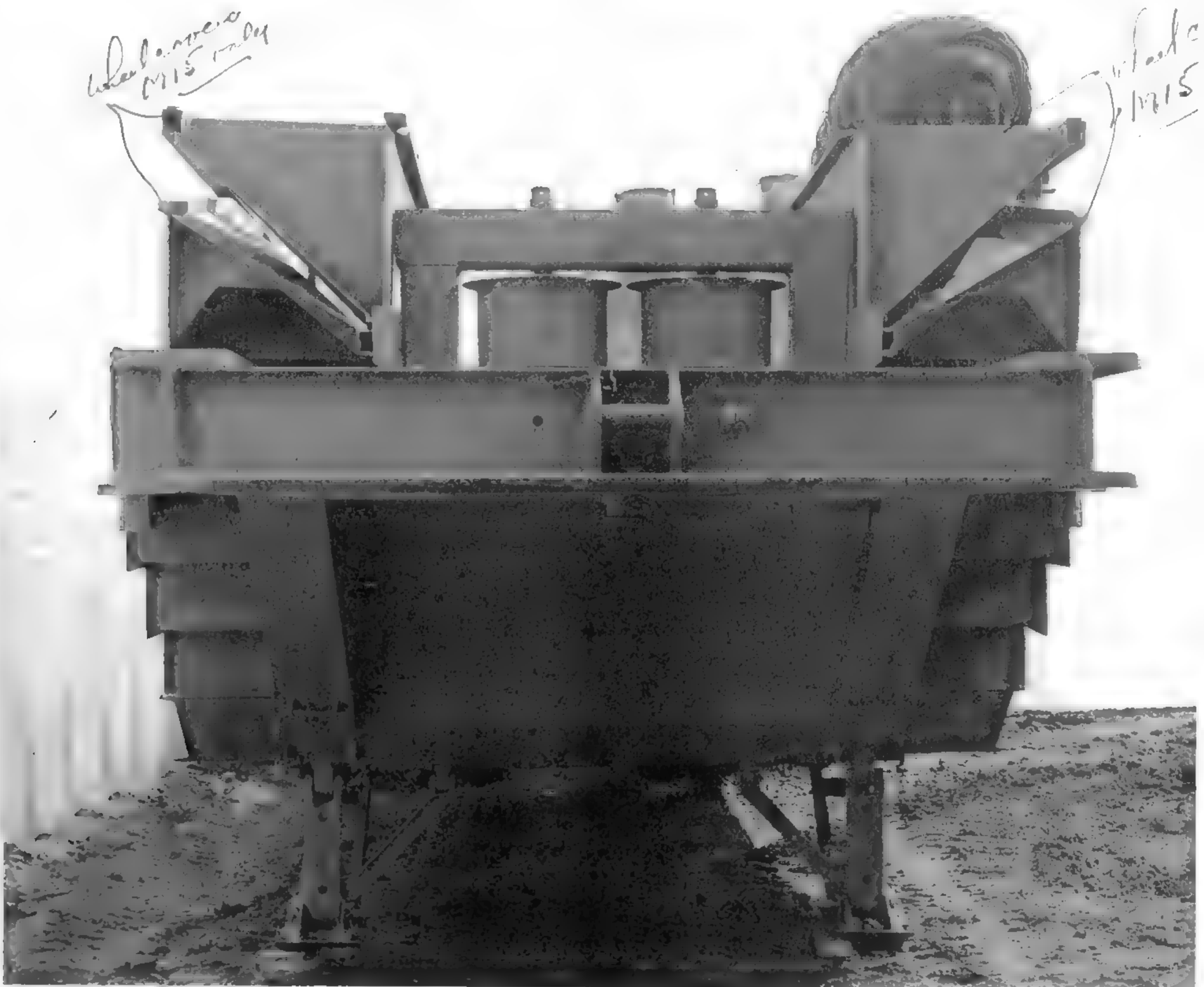
This view of the pilot M15A1 shows the large cable guide rollers at the front of the trailer. (U.S. Army photo)
